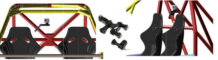
For « Pen » type cameras, it can be mounted on the front upright of the roll cage, the control unit must be fixed on the floor, behind the seats.
