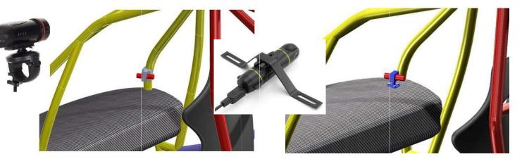
Only « Pen » type cameras will be accepted outside the car, positionned inside the perimeter of the car. Fixation must be from a mechanical type, and if a support is needed, it cannot exceed 40 mm height. Control unit must be fixed on the floor, behind the seats for touring cars or under the seats for the twin seaters. Fixation must be from a mechanical type, tape or velcro are forbidden.
